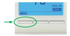
2. Press ⊗ or ⊗ to highlight the **Programming** menu item. Then press ⊚ (Action button) to enter the Programming Menu.
